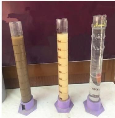
a) Sieve analysis and hydrometer test
