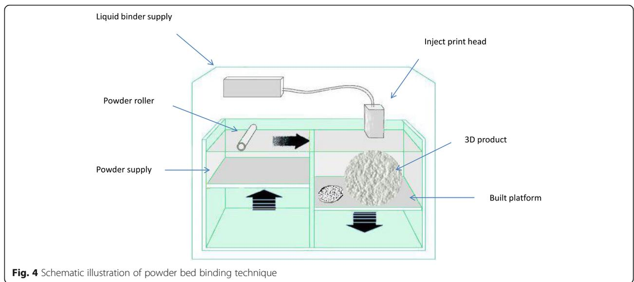
**Fig. 4** Schematic illustration of powder bed binding technique
