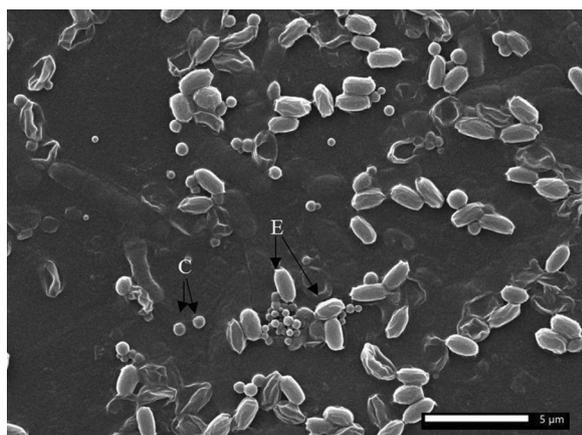
**Fig. 1** Scanning electron microscopy images of the *Bv5* strain, showing ellipsoidal spores and round proteins not attached to the spores. (Captions: C, Crystals; E, spores)
