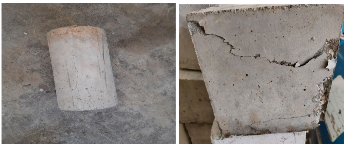
Fig. 7 Mode of failure of specimens
