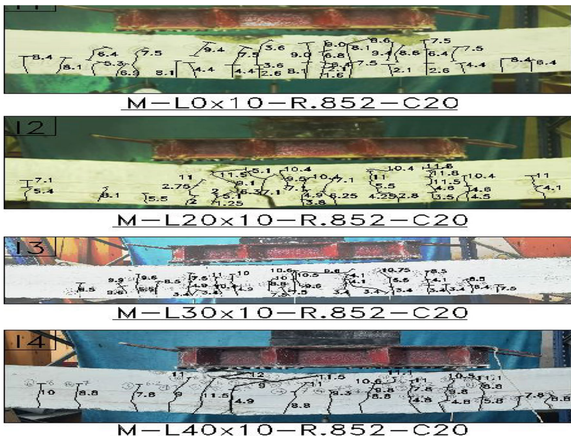
Fig. 11 The crack pattern for group (I)
