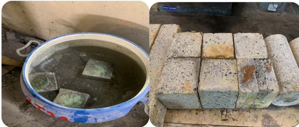
Fig. 14 Acid attack test
