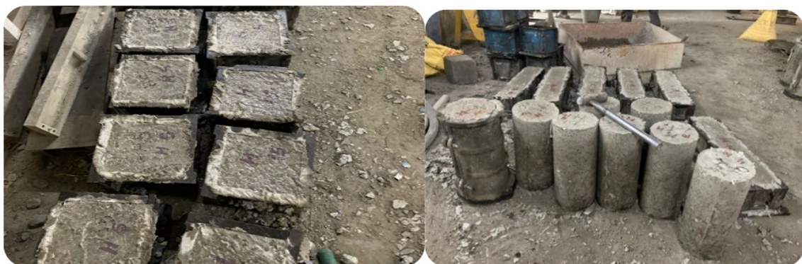
Fig. 7 a Concrete cubes and b concrete cylinders
