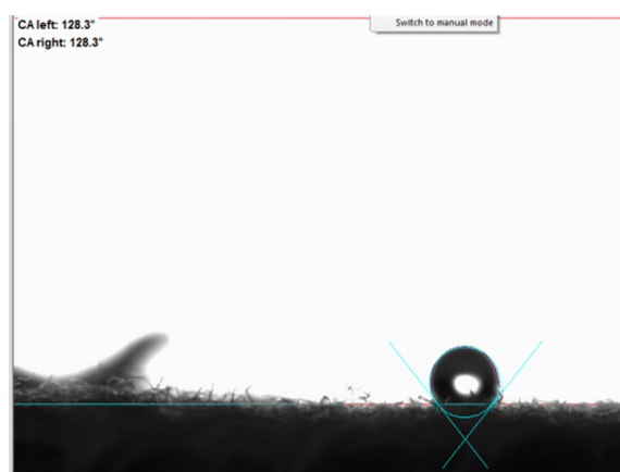
Fig. 5 Contact angle of the blank linen fabric
