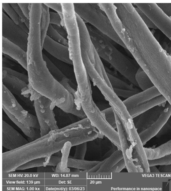
Fig. 7 Illustration of the scanning electron microscope image for the treated printed linen fabrics, respectively
