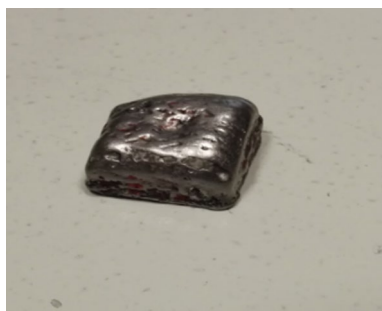
Fig. 7 Laser-Deposited AlCoCrFeNiCu High Entropy Alloy Sample
