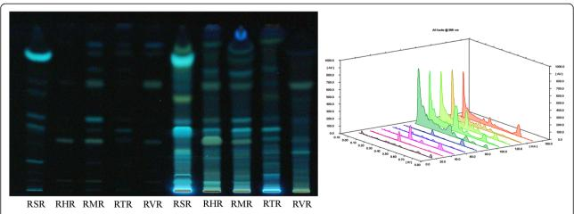
**Fig. 1** HPTLC profile of sequential n-hexane and chloroform extracts of various *Rauvolfia* species. Tracks: 1-5, n-hexane extracts; 6-10 chloroform extracts: RSR: *R. serpentina* root, RHR: *R. hookeri* root, RMR: *R. micrantha* root, RTR: *R. tetraphylla* root, RVR: *R. verticillata* root
