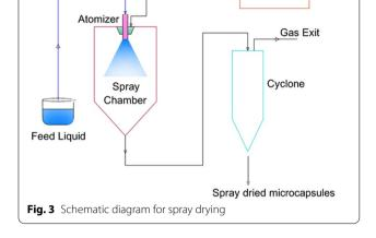
size depends on the physical properties of feed solution including surface tension, viscosity and density, pressure drop inside the nozzle and the velocity of the spray. The atomized droplet size distribution and velocity of the droplets also determine the residence time and drying rate [39].
